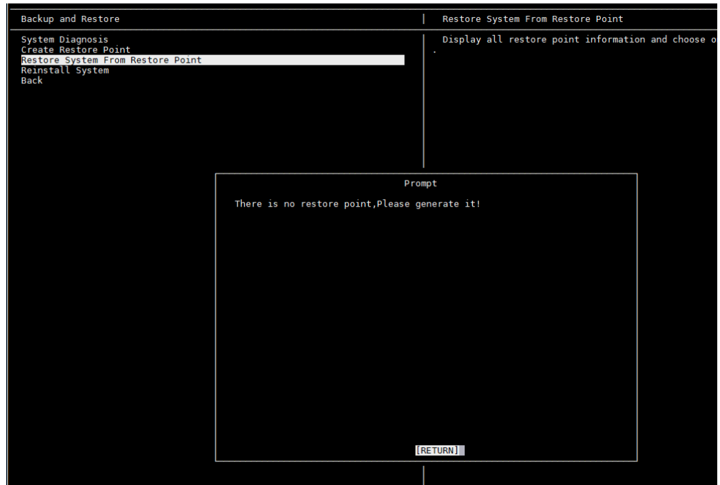
Figure A-19 Console-based management — restoring the system using a restore point
