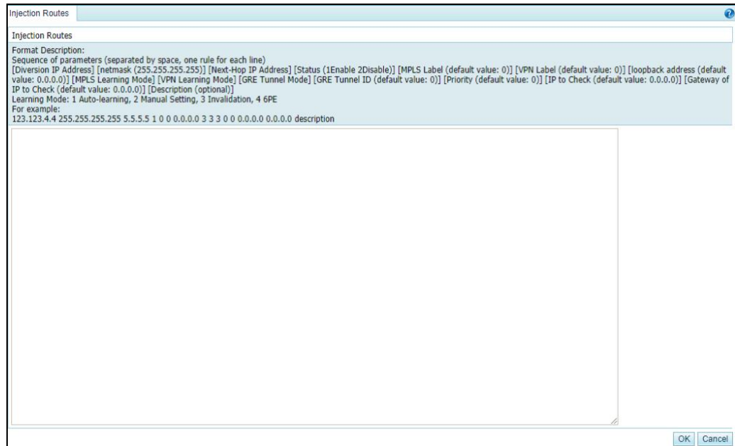
Figure 6-22 Creating injection routes in batches
