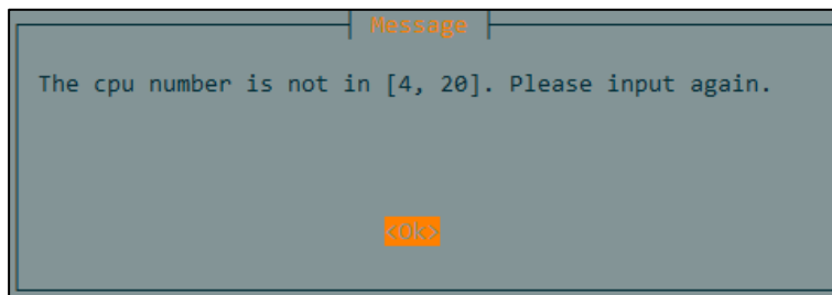
Figure 4-40 Automated deployment: typing the number again if it is outside the valid range
