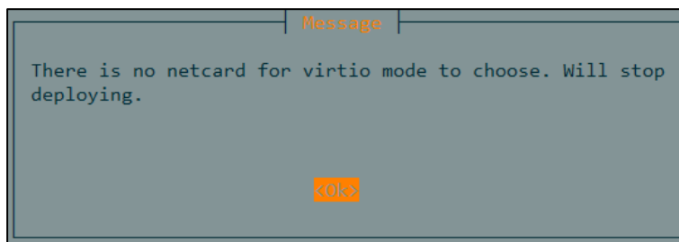
Figure 4-64 Automated deployment: no NICs available for common mode
