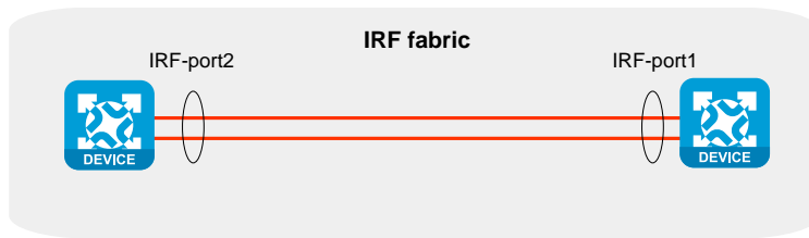
Figure 4 Connecting IRF physical interfaces
