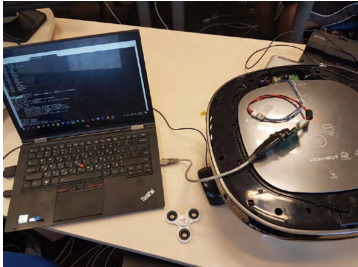
Figure 3-9 Access to the file system of an LG home-bot vacuum cleaner via the console port
