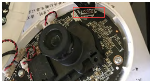
Figure 3-8 Console port pins of a camera
